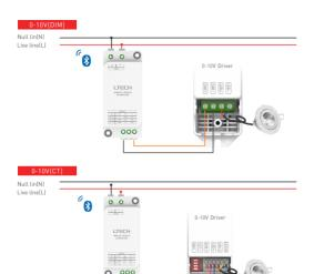
\* When it outputs 0-10V signals, this module can connect to a maximum of 100 LTECH 100 drivers on one circuit. If it connects to drivers from other brands, the number of connected drivers depends on the actual test.
